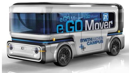
The e.GO Mover. The Mover is an universally expandable and deployable minibus, which can be equipped both for local public transport as well as for private and commercial transport use.
